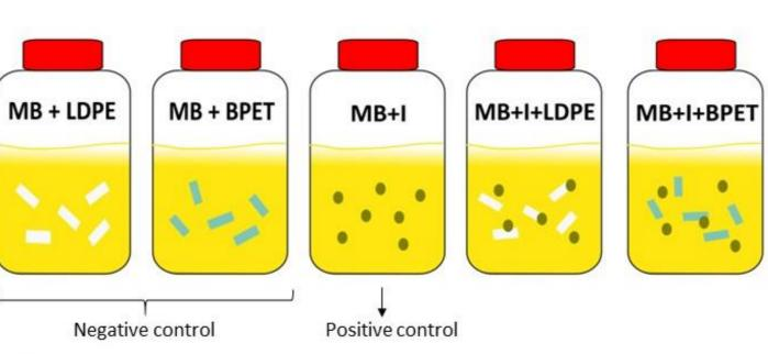
**Figure 2**. Scheme of the experimental conditions of the biodegradation experiment, in which 10 particles of each polymer (LDPE or BPET), were inoculated (10%) with different marine bacterial consortium. A negative and positive control were used, where either no inoculum, or no MPs were added, respectively. I stands for inoculum; MB for marine broth; LDPE for low-density polyethylene; and BPET for biodegradable polyethylene terephthalate.
