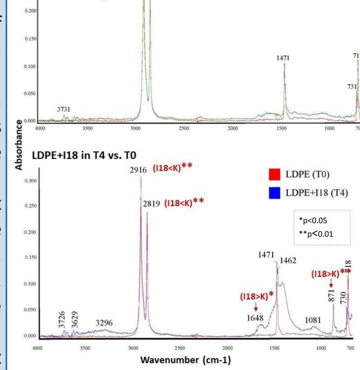
Figure 5. Spectral profile of LDPE, as determined by ATR-FTIR. The plot shows the results of the spectra spectrum of the control (LDPE-K, on the top) and the sample with the bacterial inoculate (LDPE-I18, on the bottom) at T4, superimposed to the spectrum of LDPE microplastics at the beginning of the experiment (T0).
