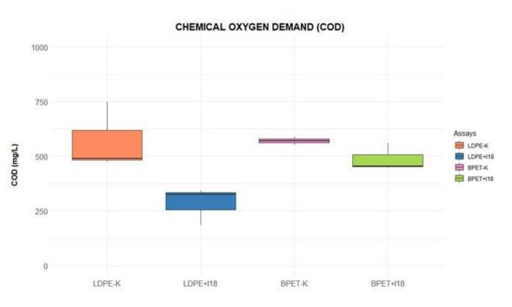
Figure 7. Representation of COD measured at the end of the experiment (after 45 days of incubation) for 5 LDPE and BPET particles. K stands for the controls and I18 for the samples inoculated with marine bacteria (inoculum 18).
