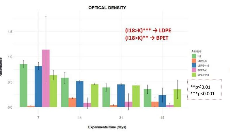
Figure 3. Results of the measurement of the optical density (at 600 nm) – as indicative of bacterial growth – throughout time for both polymers. Experimental time is shown in days. K stands for the controls and 118 corresponds to the bacterial consortium inoculated in the test samples.
